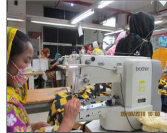
Photo of non-conformity Eye guard displaced at bartack machine.JPG
